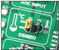
Figure 14-4: DS1820 is connected to the microcontroller via the RD0 pin
