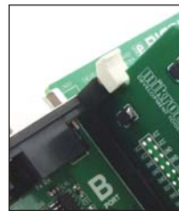
Extraction levers used for fixing MCU card in the 'closed' position
