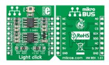
Light Click" is an accessory board in mikroBUS" form factor. It's a compact and easy solution for adding light sensor to your design. It features PD15-22C-TR8 PIN photodiode, MAX6106 voltage reference and MCP3201 ADC with SPI interface. Light Click" communicates with the target board microcontroller via mikroBUS" SPI (MISO, SCK, CS) and AN lines. The board is designed to use 3.3V and 5V power supply. LED diode (GREEN) indicates the presence of power supply.
