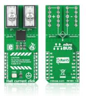
Hall current click<sup>™</sup> is a high precision current sensor. It carries a galvanically isolated TLI4970-D050T4 miniature magnetic digital current sensor that utilizes the Hall effect to measure electric current. The board carries two EXTreme ZPower connectors to connect the conductor. The sensor readings are sent to the target board through the **mikroBUS<sup>™</sup>** SPI (SDO, SCK, and CS) lines. The board uses a 3.3V power supply only.
