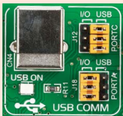
Figure 8-2: USB enabled on PORTC
