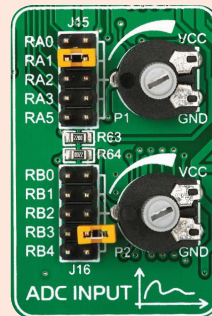
Figure 17-1: use J15 and J16 jumpers to connect analog input lines with potentiometers P1 and P2
