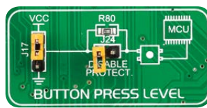
Figure 10-5: Button press level jumper (J17)
