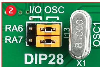
Figure 4-7: RA6 and RA7 connected to X1 quartz-crystal
