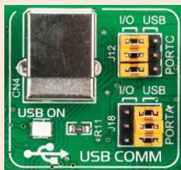
Figure 8-3: USB enabled on PORTA
