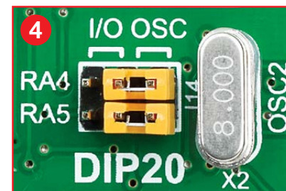
Figure 4-9: RA4 and RA5 connected to X2 quartz-crystal
