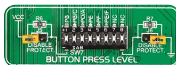
Figure 10-6: Button press level DIP switch (tri-state)
