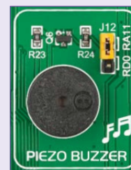
Figure 19-2: Use jumper J12 to connect Piezo buzzer on RDO or RA11 pin
