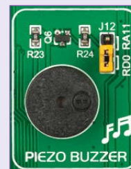
Figure 19-2: Use jumper J12 to connect Piezo buzzer on RDO or RA11 pin
