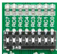
Figure 6-2: Tri-state DIP switch on PORTC
