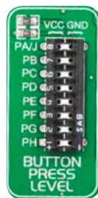
Figure 6-5: Button press level DIP switches (tri-state)
