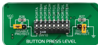
Figure 6-5: Button press level DIP switch (tri-state)
