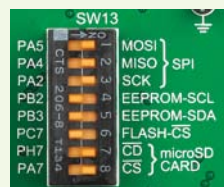
Figure 15-2: enabling microSD card commu- nication lines
