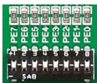
Figure 6-2: Tri-state DIP switch on PORTE
