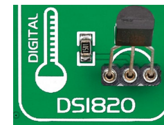
Figure 23-3: DS1820 correctly placed in socket
