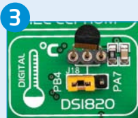
Figure 14-3: DS1820 connected to PB4 pin
