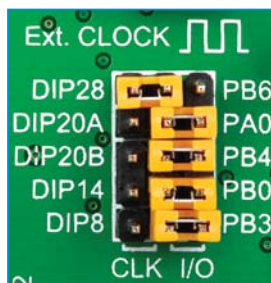
Figure 4-6: Position of the jumpers for DIP28
