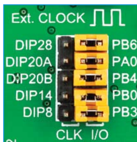
Figure 4-5: Position of the jumpers for DIP40x
