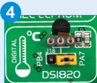
Figure 14-4: DS1820 connected to PA7 pin
