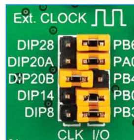
Figure 4-8: Position of the jumpers for DIP20B
