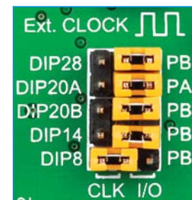
Figure 4-10: Position of the jumpers for DIP8
