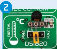
Figure 14-2: DS1820 placed in socket
