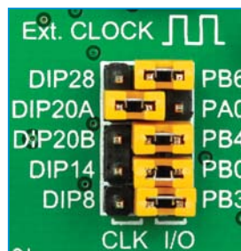
Figure 4-7: Position of the jumpers for DIP20A
