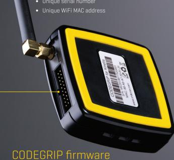
The CODEGRIP device is equipped with the target MCU connector, which contains JTAG/SWD and power supply pins. This connector is used to interface the CODEGRIP device with the target MCU, allowing it to perform programming and debugging operations, to provide the power supply for the target MCU, and to be used as the power input when the CODEGRIP device is powered from the connected development board.
