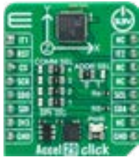
Accel 29 Click Based on the ADXL314, a three-axis \pm 200g accelerometer from Analog Devices. MSRP – $27 00 MIKROE-5671
