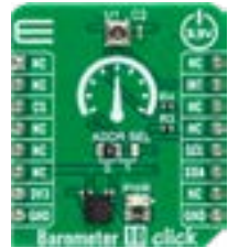
Barometer 10 Click With the LPS28DFW, an ultra-compact piezoresistive absolute pressure sensor from STM. MSRP – $24 00 MIKROE-5601
