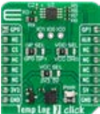
Temp-Log 7 Click Features the TMP1826, a 1-Wire ® compatible digital output temperature sensor from TI. MSRP – $9 00 MIKROE-5598
