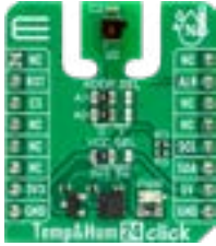
Temp&Hum 24 Click Carries the HDC3021, humidity and temperature sensor Texas Instruments. MSRP – $12 00 MIKROE-5651
