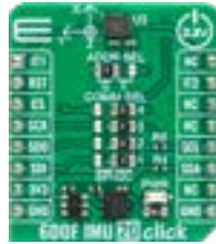
6DOF IMU 20 Click Features the BMI323, a high-performance, low-power IMU from Bosch. MSRP – $17 00 MIKROE-5606
