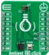
Ambient 23 Click With the VEML3235SL, an advanced ambient light sensor from Vishay. MSRP – $11 00 MIKROE-5701
