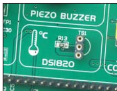
Figure 6-1: DS1820 connector (DS1820 is not connected)
