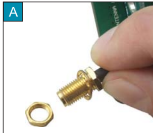
Figure 9-4: Screwing cable into antenna holder
