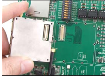
Figure 9-2: Connecting Telit's GM862 module
