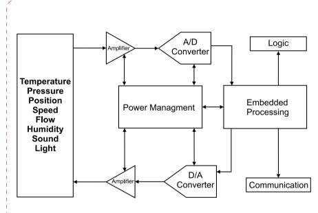
Figure: Signal Chain in an Electronic System
