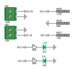
Figure D.18: Main power supply
