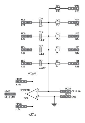
Figure D.2: OP-Amp 1B connected in inverting configuration
