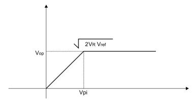
Figure 8.2: Input-Output Characteristics of AGC/AVC
