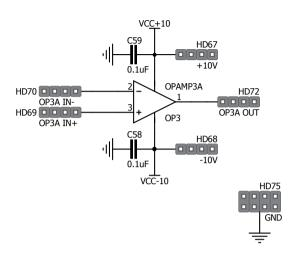
Figure D.5: OP-Amp 3A can be used in unity gain configuration or any other custom configuration
