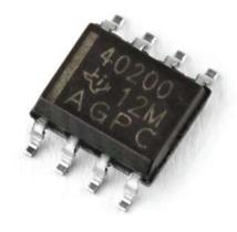
Figure A.4: TPS40200 - DC/DC Controller
