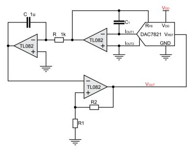
Figure 14.1: Circuit for Digital Controlled Oscillator
