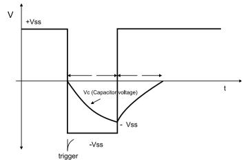
Figure 2.6: Monostable Multivibrator and its outputs
