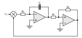
Figure 6.3: Voltage-Controlled Oscillator (VCO)
