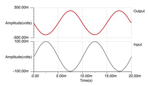
Figure 13.3: Simulation output of digitally controlled gain stage amplifier when the input pattern for the DAC was selected to be 0x800
