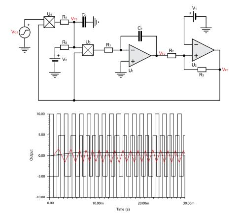
Figure 7.2: Sample output waveform for the Phase Locked Loop (PLL) Experiment
