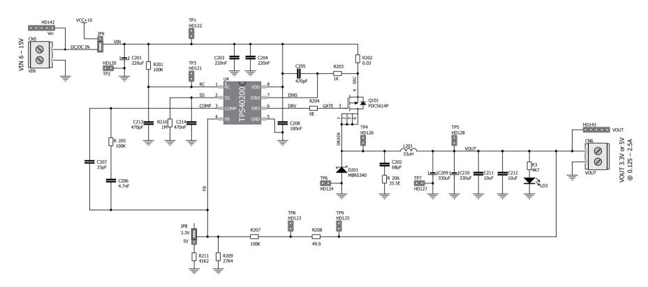
Figure 12.1: Schematic of the on-board EVM
