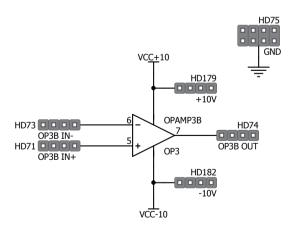
Figure D.6: OP-Amp 3B can be used in unity gain configuration or any other custom configuration
