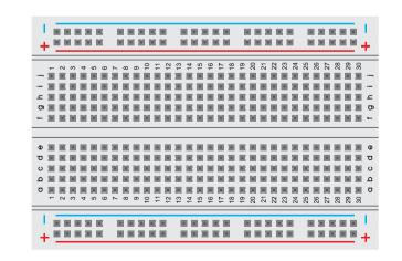
Figure D.19: General purpose area (2.54mm / 100mills pad spacing)
