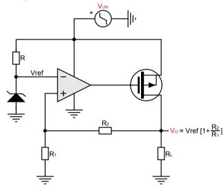
Figure 10.1: Low Dropout Regulator (LDO)
