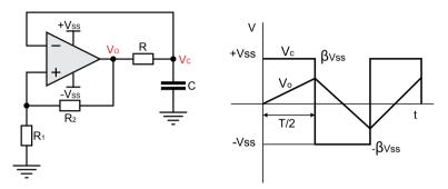
Figure 2.4: Astable Multivibrator and its characteristics
