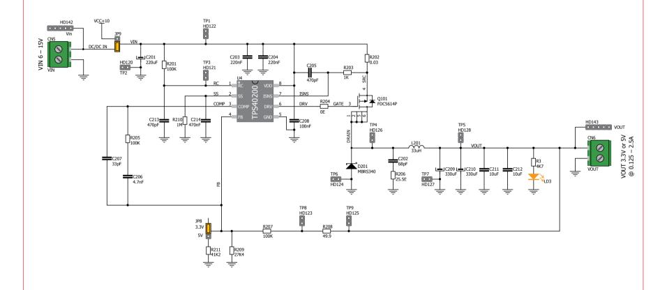
Figure D.12: Connections for TPS40200 Evaluation step-down DC/DC converter
