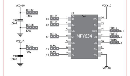
Figure D.9: Connections for analog multiplier MPY634 - SET III
