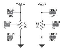
Figure D.17: Trimmer-potentiometers
