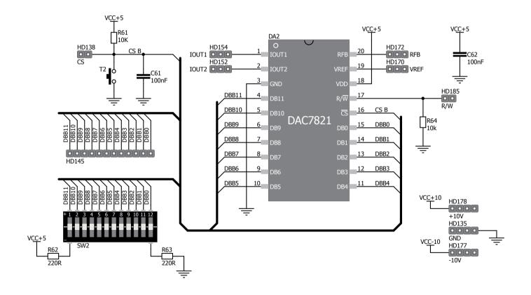
Figure D.11: connections for analog-to-digital converter DAC7821 - DAC II
