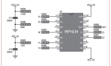
Figure D.7: Connections for analog multiplier MPY634 - SET I
