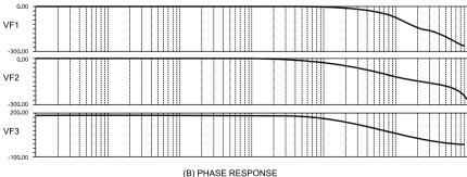
Figure 1.7: Frequency Response of Negative Feedback Amplifiers
