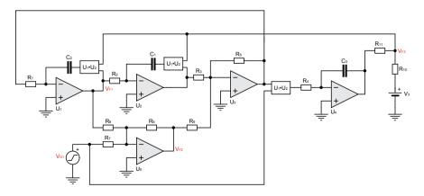
Figure 5.2: A Self-Tuned Filter based on a Voltage Controlled Filter or Voltage Controlled Phase Generator
