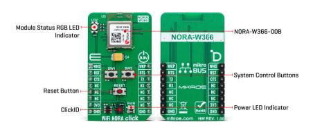
Pre-flashed with u-connectXpress software, the NORA-W366-00B module simplifies end-product integration and accelerates time-to-market. It includes a TCP/IP stack for both point-to-point and point-to-multipoint use cases and ensures secure communication with cloud-based services through support for TLS encryption and MQTT protocols. The module also offers robust security features, including WPA2/WPA3, WiFi enterprise security, and Bluetooth LE secure connections.
