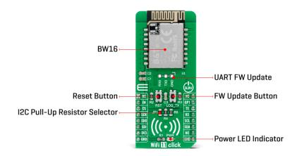
WiFi 11 Click communicates with the MCU using the UART interface at 57600 bps as its default communication protocol, but the user can also use other interfaces, such as SPI and I2C if he wants to configure the module and write the library himself. A jumper JP1 on this Click board also enables the necessary pull-up resistors on the SCL and SDA lines of I2C communication.
