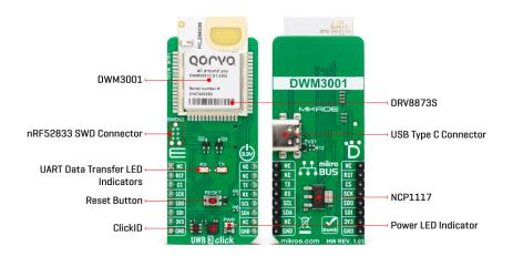
The DWM3001 UWB transceiver also incorporates the LIS12DH, a low-power three-axis linear accelerometer from STMicroelectronics. It is necessary as RTLS tags commonly use accelerometers to initiate UWB ranging only when a tag moves so that battery life can be extended by staying in the lowest power mode by default. Near-field communication type 2 (NFC-A) can be used by adding an NFC antenna to the TP1 and TP2 pads.
