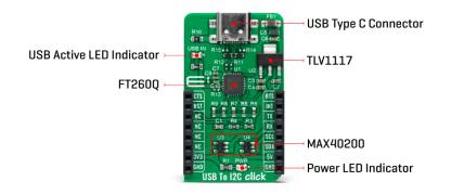
This Click board<sup>™</sup> can communicate with MCU via UART or I2C interface. The FT260Q uses the UART interface with commonly used UART RX and TX pins and hardware flow control pins UART CTS and RTS (Clear to Send and Ready to Send) to transmit and exchange data with the host MCU or using the I2C interface, which can also act as a Master with a maximum I2C bus speed of up to 3.4Mbit/s. These two interfaces exist concurrently and can be selected independently according to the application.
