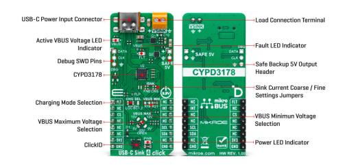
The CYPD3178 on the USB-C Sink 4 Click supports multiple charging protocols. When connected to a non-PD charger, it can negotiate with any legacy charging protocol supported by the sink device. The CHG SEL jumper allows users to configure the supported protocols. The jumper is set to the LGC position by default, enabling support for all legacy charging protocols. However, by switching the jumper to the BC1.2 position, the device limits its operation to the BC1.2 charging protocol only.
