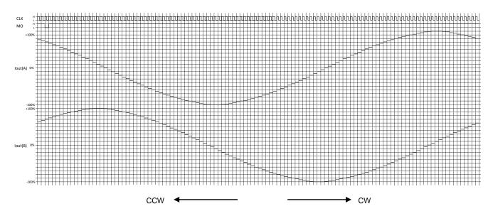
MO is a waveform of the pin output in pull-up state.
