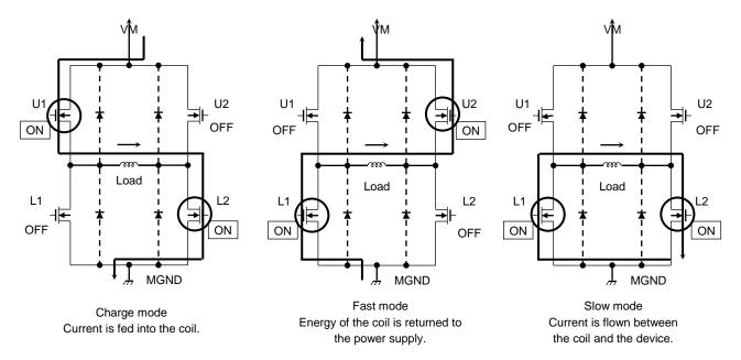
\*A shoot through-current prevention period (dead time) is provided inside the device to prevent shoot through-current when switching outputs.
