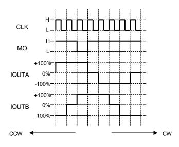
MO is a waveform of the pin output in pull-up state.
