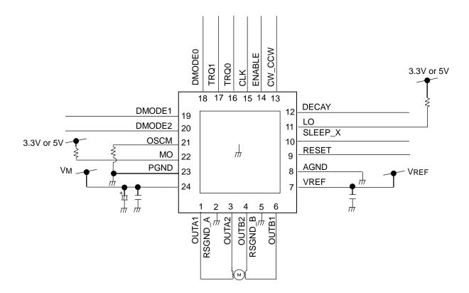
Heat dissipation PAD (the center part) on the back of the package is recommended to connect to the ground of the board for improved heat dissipation.
