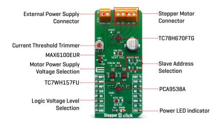
Stepper 8 Click can operate a bipolar stepper motor in full, half, quarter, 1/8, 1/16, 1/32, 1/64, 1/128 step operation. Thanks to internal safety features, such as thermal shutdown (TSD), over current (ISD), motor load open (OPD) and under voltage lockout(UVLO), this Click board<sup>™</sup> is perfectly suited for rapid development of various stepper motor applications.
