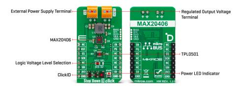
As mentioned, the Step Down 9 Click uses the TPL0501 and its 3-Wire SPI serial interface to communicate with the host MCE, supporting clock frequency of up to 25MHz. The voltage quality can be monitored by observing the PGOOD signal over the PG pin of the mikroBUS™ socket. The enable EN pin is an input for circuit activation, active with a HIGH logic state.
