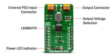
The output voltage supervisor manages the reset phase for any digital load ( $\mu$ C, FPGA). The RST open collector output can also implement output voltage sequencing during the power-up phase. The synchronous rectification, designed for high efficiency at medium - heavy load, and the high switching frequency capability make the size of the application compact. Pulse by pulse current sensing on both power elements implements an effective constant current protection.
