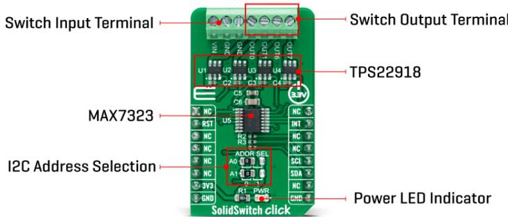
This Click board™ is designed to operate from an external supply voltage range from 1V to 5.5V. The TPS22918 works regardless of power sequencing order. The order in which voltages are applied to the VIN terminal and ON pin of the load switch will not damage the device as long as the voltages do not exceed the absolute maximum operating conditions.
