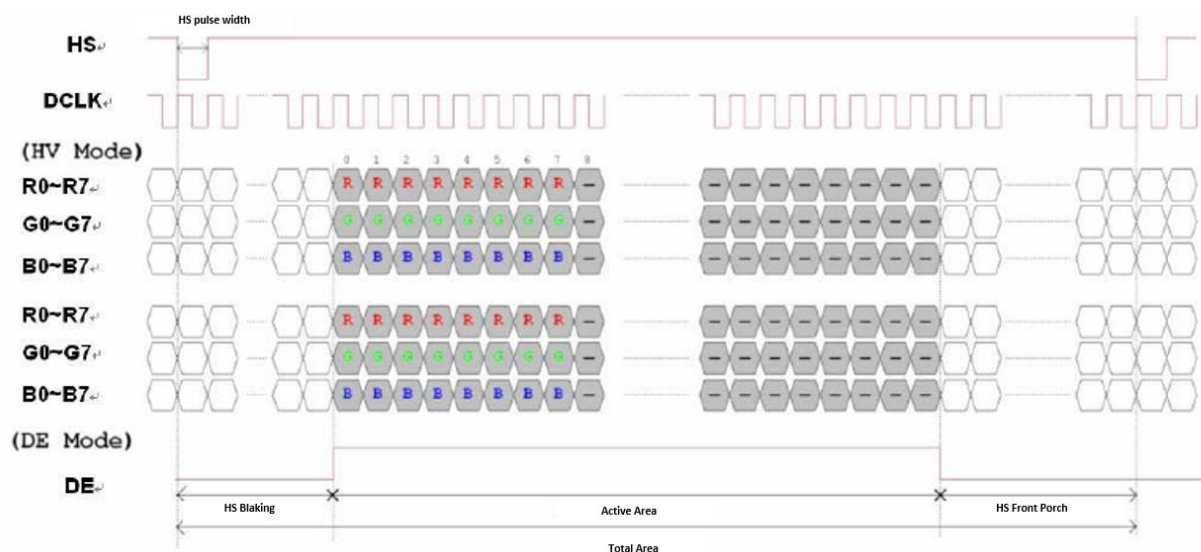
Figure 5. Horizontal input timing diagram
