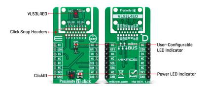
The VL53L4ED uses STMicroelectronics' FlightSense technology, allowing it to measure absolute distances regardless of target color or reflectance. It includes a SPAD (single photon avalanche diode) array, enhancing its performance across ambient lighting conditions and various cover glass materials. Additionally, the sensor integrates a VCSEL (vertical-cavity surface-emitting laser) that emits an invisible 940nm IR light, certified as Class 1 eye-safe.
