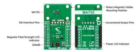
The MA735 uses integrated Hall devices to detect the magnetic field, while the angle is measured using MPS's proprietary Spinaxis™ method. This method is based on phase detection and digitizes the direction of the field directly, generating a sinusoidal signal with a phase that represents the angle of the field. The angle is obtained from a signal by a time-to-digital converter, and the digital number proportional to the magnetic field is delivered at a rate of 1MHz.
