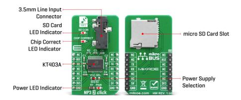
On the MP3 2 Click, KT403A serves as a brain. It is complete SOC, which integrates16-bit MCU, audio decoder, and a 24-bit DSP. It also integrates the complete SD card interface and therefore, this click board contains the connector onboard for an external micro SD card. Thanks to that, the user can insert a fair amount of memory if the long, continuous playback time is needed.
