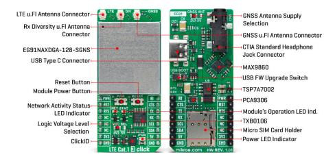
Communication between the EG91NAXDGA-128-SGNS and the host MCU is made through a UART interface, using standard UART RX and TX pins and hardware flow control pins (CTS/RTS/RI - Clear to Send/Ready to Send/Ring Indicator) for efficient data transfer. The module defaults to a communication speed of 115200bps, allowing for seamless data exchange over <u>AT commands</u>. Notably, this telematics version of the module also features an audio interface, which can be accessed via the I2C interface.
