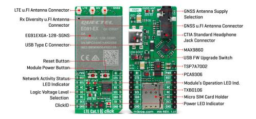
Communication between the EG91EXGA-128-SGNS and the host MCU is made through a UART interface, using standard UART RX and TX pins and hardware flow control pins (CTS/RTS/RI - Clear to Send/Ready to Send/Ring Indicator) for efficient data transfer. The module defaults to a communication speed of 115200bps, allowing for seamless data exchange over AT commands. Notably, this telematics version of the module also features an audio interface, which can be accessed via the I2C interface.
