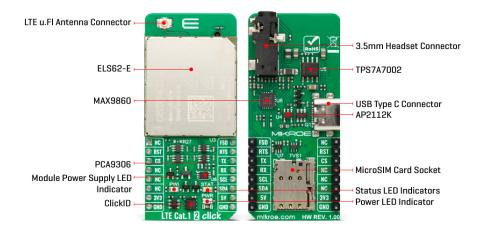
The ELS62-E supports a digital audio interface (DAI) employed as a pulse code modulation interface (PCM). The PCM interfaces the MAX9860, a 16-bit mono audio voice codec from Analog Devices. It supports a low-noise microphone input, mono amplifier, automatic microphone gain control and noise gate, and more. The audio codec can output 30mW into a  $32\Omega$  earpiece with a microphone connected over the 3.5mm audio jack.
