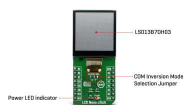
The display used for this click, the LS013B7DH03 LCD, is a 1.28", 128x128 pixels monochrome display, with a 3-wire SPI interface. Apart from the SPI interface, the display requires a 3.3V power supply, and 3 extra pins named EXTMODE, EXTCOMIN and DISP. The SPI protocol consists of three modes. At the start of each SPI transfer, a mode command (1 byte) is sent first. The modes are:
