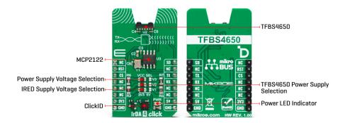
To communicate with the host MCU, IrDA 4 Click uses MCP2122 and its onboard clock
