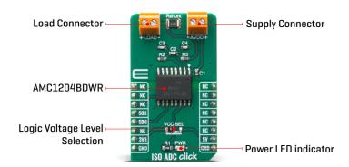
The ISO ADC Click perform current measurement on LOAD connector, the AMC1204BDWR measure the differential input signal VIN = (VINP - VINN) on two ends of the shunt resistor, against the internal reference of 2.5 V using internal capacitors that are continuously charged and discharged. The current measurement can't be possible without external power supply on AVDD connector.
