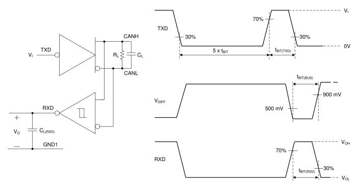
Figure 21. CAN FD Timing Parameter Measurement
