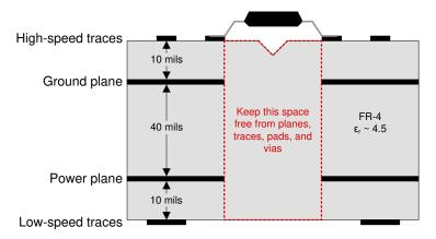
Figure 34. Recommended Layer Stack
