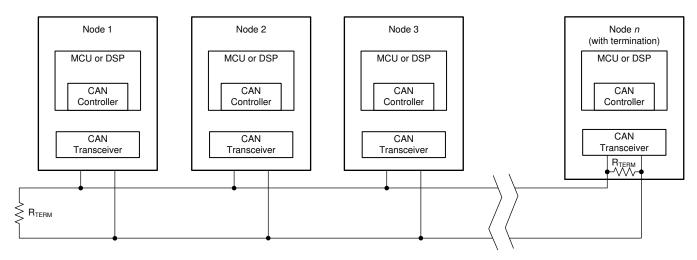
Figure 30. Typical CAN Bus
