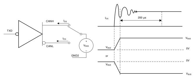
Figure 23. Driver Short-Circuit Current Test Circuit and Waveforms
