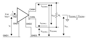
Figure 15. Driver Voltage, Current and Test Definitions
