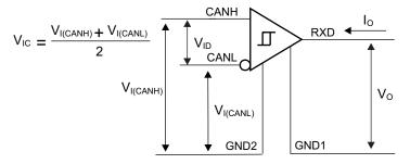
Figure 18. Receiver Voltage and Current Definitions
