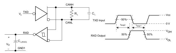
Figure 20. t<sub>LOOP</sub> Test Circuit and Voltage Waveforms
