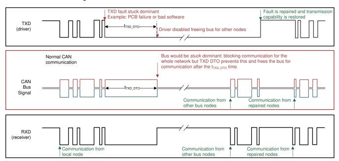
Figure 27. Example Timing Diagram for TXD DTO
