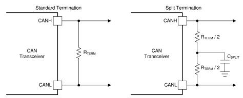
Figure 31. CAN Bus Termination Concepts
