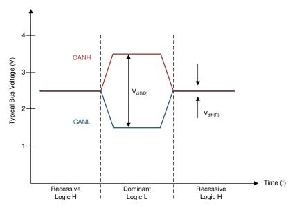
Figure 25. Bus States (Physical Bit Representation)
