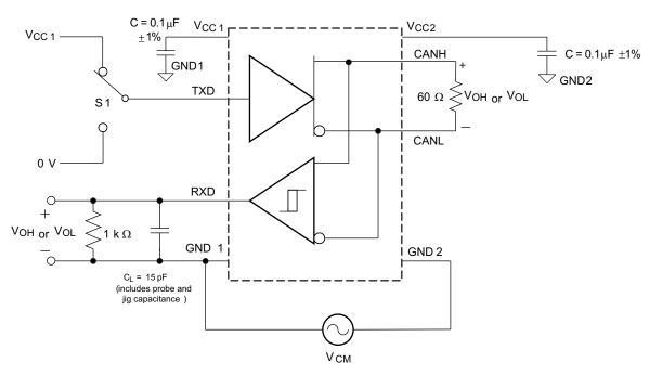
Figure 24. Common-Mode Transient Immunity Test Circuit
