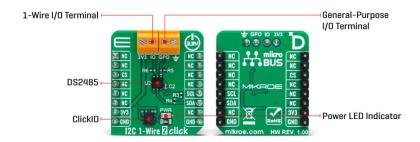
Upon receiving commands and data, the DS2485's input/output management unit takes over the execution of crucial 1-Wire operations such as the reset/presence-detection cycle, byte reading and writing, block reading and writing, single-bit read/write operations, executing triplets for ROM search activities, and handling complete command sequences for 1-Wire authenticators—all without the need for continuous host processor intervention.
