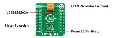
As a result of this very effective drive, the vibration is as powerful as possible using minimal energy compared to classical solutions. It also ignores the deviation of resonance frequency thanks to auto-tuning function. This function can increase the perceived vibration force by over 20%, making it far more efficient than conventional haptic driving solutions. They require minimal power but are capable of maintaining a high level of vibration.
