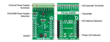
The TCAL6408 supports independent logic and power supplies. The logic voltage is supplied via the 3.3V mikroBUS<sup>™</sup> power rail, while the main power can be selected between 3.3V from the mikroBUS<sup>™</sup> or an externally provided supply through the VIN terminal, with a range of 1.08V to 3.6V. The main power selection is managed by the VCCP SEL jumper, allowing users to set the appropriate power source for the TCAL6408 based on their application's requirements.
