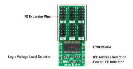
Configuration and output register settings are storable as user defaults in a dedicated section of the EEPROM. If user defaults were stored in EEPROM, they are restored to the ports at Power-Up. The EEPROM is byte readable and supports byte-by-byte writing. A pin 3 of the Port 2 on this Click board  $^{\text{m}}$  can be configured as an EEPROM Write Disable (WD) input that blocks write operations when set high. The configuration registers can also disable EEPROM operations.
