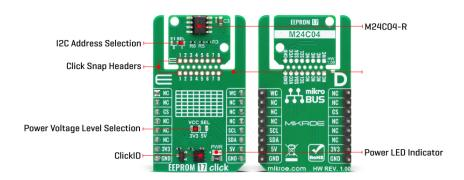
The entire memory array can be write-protected to safeguard critical data against unintended modifications. The M24C04-R offers exceptional endurance with more than 4 million guaranteed write cycles per memory cell and ensures long-term data integrity with a data retention period exceeding 200 years.
