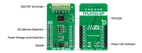
DIGI POT 14 Click uses a standard 2-Wire I2C interface to communicate with the host MCU and supports Standard and Fast mode with up to 400kHz of clock frequency. The I2C address can be set over the ADDR SEL jumpers, where 0 is set by default. Both potentiometers' high, low, and wiper pins are tied to screw terminals, properly labeled as A and B sides.
