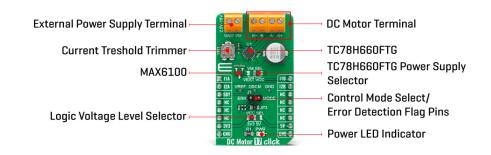
The TC78H660FTG possesses two operational modes, IN Input Mode and PHASE Input Mode, whose selection can be achieved via headers Control Mode pin labeled as MODE. PHASE Mode represents the default mode of this Click board<sup>™</sup>, and the Control Mode is set up by the input state of the MODE pin after releasing the SBY pin. This way, the MODE pin is used as the Enable signal while the direction selection is realized via GPIO pins routed on the mikroBUS<sup>™</sup> socket.
