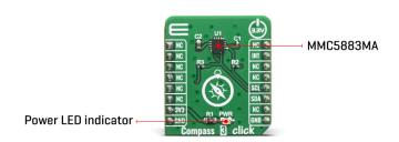
An integrated SET/RESET function provides for the elimination of error due to Null Field output change with temperature. Temperature information from the integrated temperature sensor is available over the I2C Interface.
