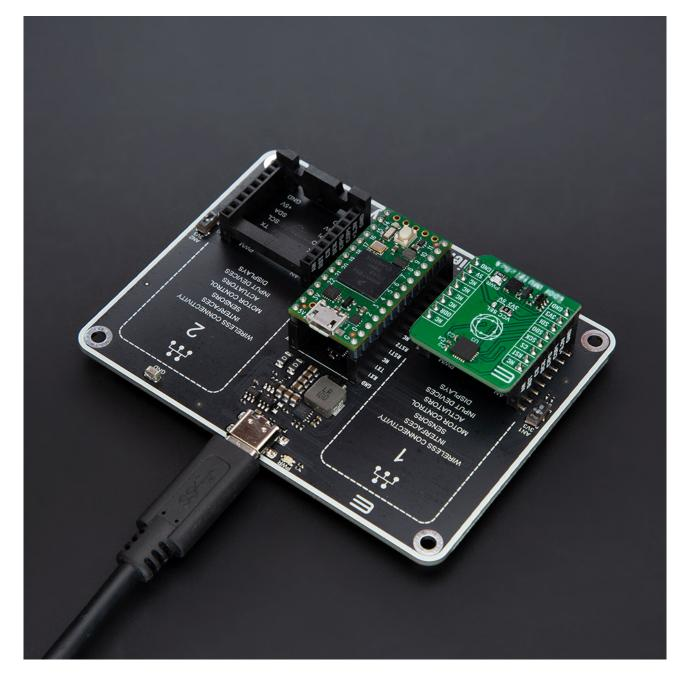
When the USB type C is connected to the Click Shield, the PWR diode will glow Blue, and at this setup, the connected Teensy 4.0 host board and all mikroBUS $^{\text{m}}$  sockets will be powered from it.
