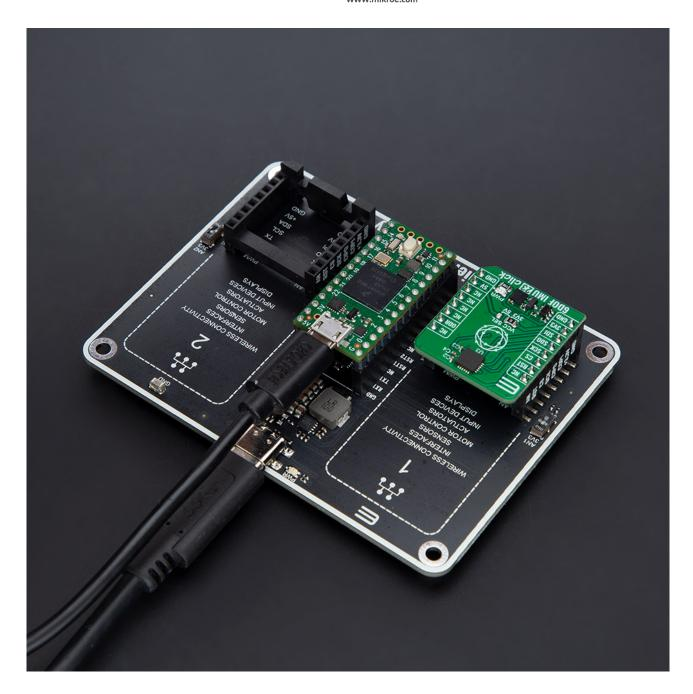
When the USB type C is connected to the Click Shield and the other USB is connected to the Teensy 4.0 board, the PWR diode will glow Cyan, and at this setup, the mikroBUS $^{\text{m}}$  sockets are powered from the Click Shield.
