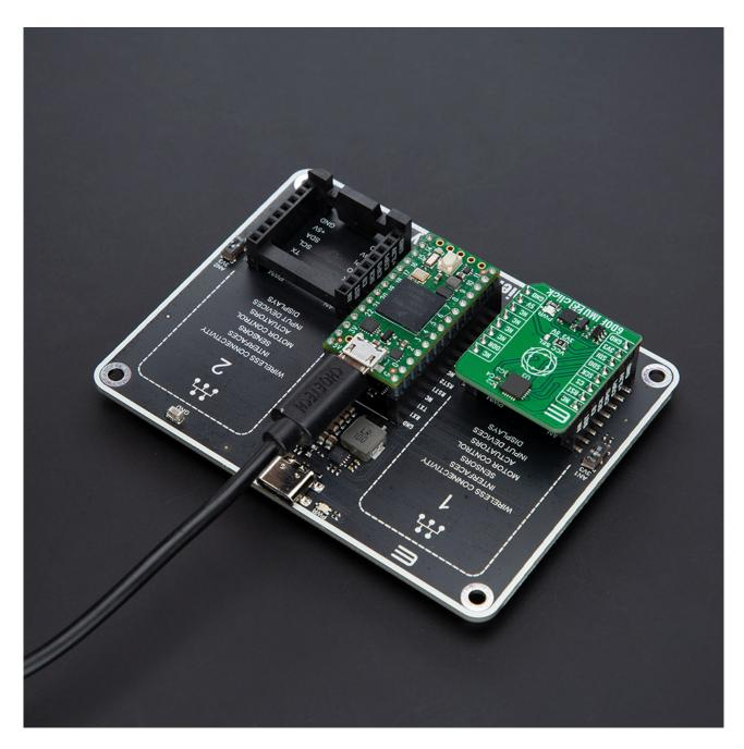
When the USB is connected to the Teensy 4.0 board, the PWR diode will glow Green, and at this setup, the Teensy 4.0 host board itself will be supplied, and it will provide power to the Click Shield, including all mikroBUS<sup>™</sup> sockets.
