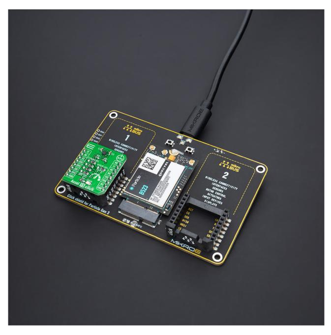
When the USB type C connector is connected to the Click shield for Particle Gen 3, the connected Click shield and mikroBUS<sup>™</sup> sockets will be powered from it.
