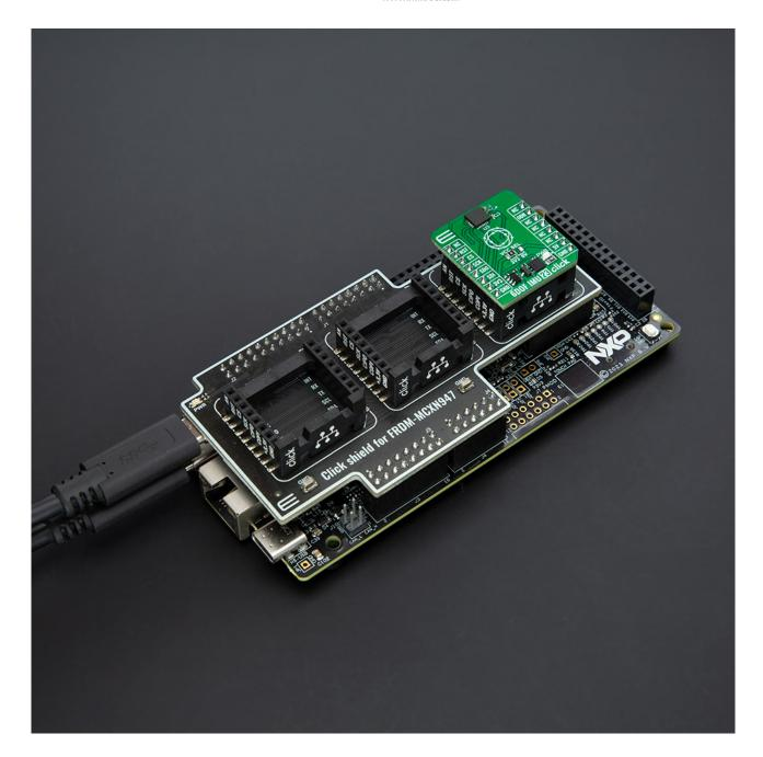
When the USB type C is connected to the Click Shield and the other USB is connected to the FRDM-MCXN947 board, the PWR diode will glow Cyan, and at this setup, the mikroBUS™ sockets are powered from the Click Shield.
