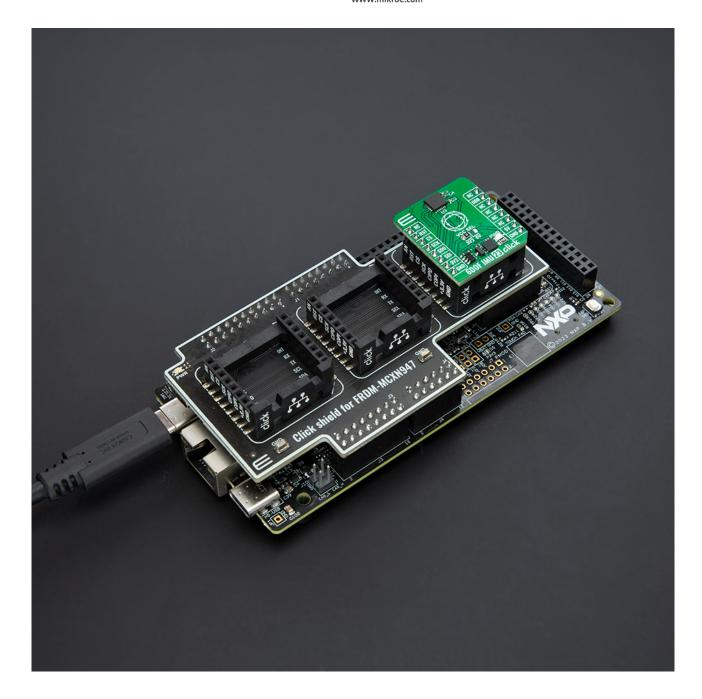
When the USB is connected to the FRDM-MCXN947 board, the PWR diode will glow Green, and at this setup, the FRDM-MCXN947 host board itself will be supplied, and it will provide power to the Click Shield, including all mikroBUS™ sockets.
