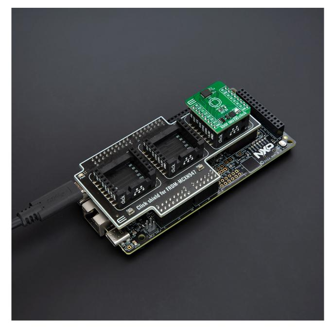
When the USB type C is connected to the Click Shield, the PWR diode will glow Blue, and at this setup, the connected FRDM-MCXN947 host board and all mikroBUS $^{\text{m}}$  sockets will be powered from it.
